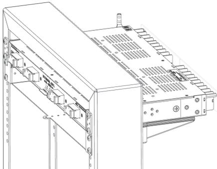
**Correct installation of a heat baffle.**
